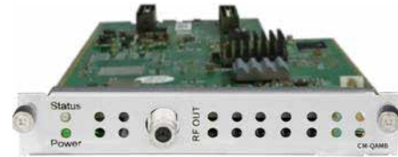
CM2-QAMB-R01/R01A: QAMB Modulation Module
