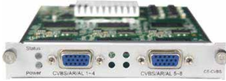
CE2-CVBS-R01: Commercial CVBS Encoder Module
