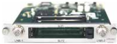
CR2-DVBS2CI-01: DVB-S/S2/S2X with CI Receiver Module
