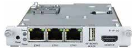
CP2-IP-00: Multi-protocol IP Module
